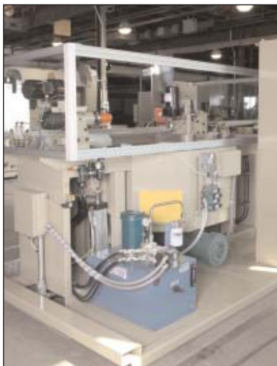
Rear view of 2SF-48RA Spindle Machine featuring Hydraulic Package supplying fluid to rotary actuary feature on spindle arms.
