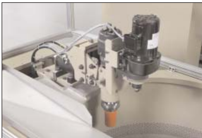
2SF-48RA Variable Speed Spindle Head in the down position for part procession in a rotating mass of abrasive media.
